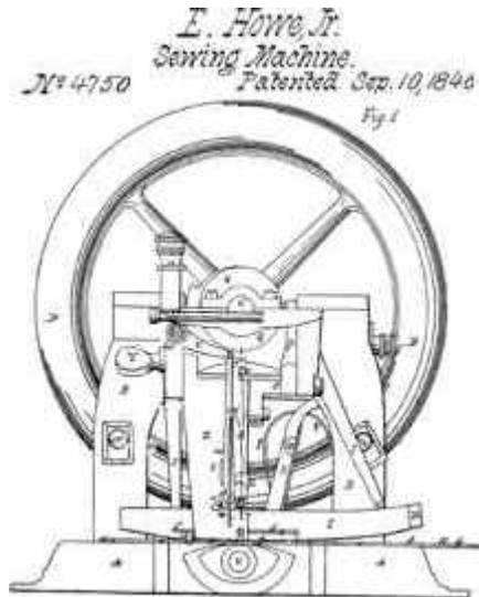
Figure 3.4: The lockstitch sewing machine of Elias Howe.
