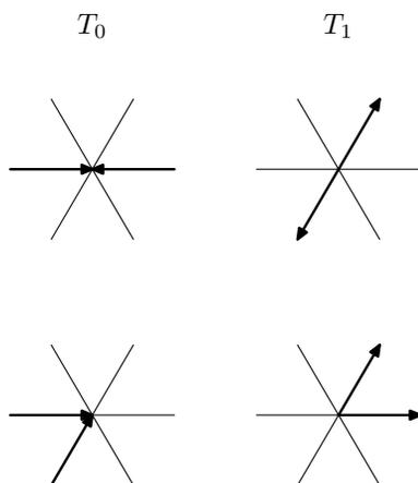
Figure 1.8: Collisions in a lattice gas: ‘Molecules’ colliding head on bounce off at  $60^\circ$  angles (above). In other cases the collision is indistinguishable from a miss (below). In all cases Newtonian momentum and energy are conserved.
